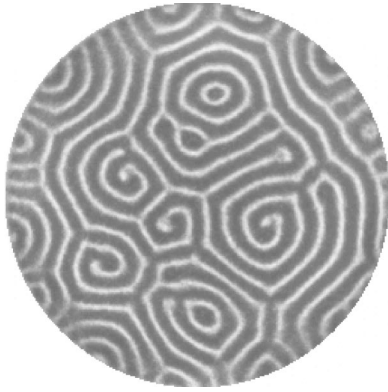
FIG. 17. A snapshot of the spiral defect chaos state in a flat-bottomed cell at N=15.4 , f=40 Hz, and \Gamma=3.13 . This pattern is time dependent and eventually evolves to a stripe pattern with defects as in Fig. 4.
