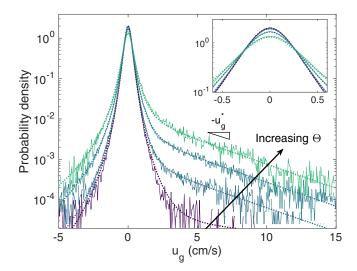
FIG. 6. The PDFs  $P(u_g)$  of grain velocities  $u_g$  (solid curves), for  $\Theta = 0.0059, 0.0232, 0.0283, and 0.0425$ . Dashed curves show fits of the data to Eq. (3). The inset shows a close-up of the same data near the core of the PDF.
