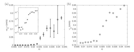
FIG. 4. (a) Mean grain velocity  $\langle u_g \rangle$  as a function of Shields number  $\Theta$ . The error bars show the standard error computed for six trials and the inset shows the same data plotted on semilogarithmic axes. (b) Standard deviation of grain velocity  $\sigma_g$  as a function of  $\Theta$ .
