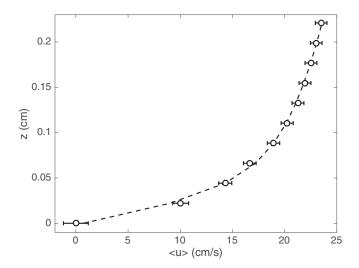
FIG. 2. Typical fluid velocity profile, as measured from the streamwise velocities u of tracer particles in the fluid. Each data point (open circles) represents a time average over all tracer particle trajectories for binned values of the height. The error bars show the standard deviation of the velocities in each bin. The dashed line is a fit following the procedure described by Rodríguez-López *et al.* [26], from which we extract the wall shear stress  $\tau_{wall}$  (see the text).
