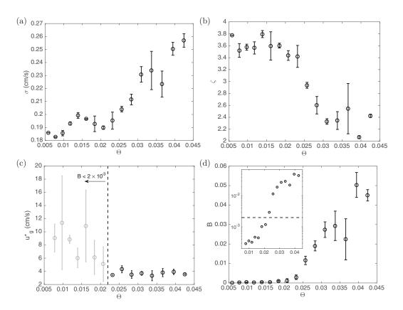
FIG. 7. Fit parameters (a)  $\sigma$ , (b)  $\zeta$ , (c)  $u_g^*$ , and (d) *B* from Eq. (3) as a function of Shields number  $\Theta$ . In all cases, the error bars are the standard error computed over six different experimental trials. We mark in (c) points (in gray) at which  $B < 2 \times 10^{-3}$ , where our fit for  $u_g^*$  is no longer physically meaningful. The inset to (d) shows the same data plotted on semilogarithmic axes, with a horizontal line at  $B = 2 \times 10^{-3}$ .
